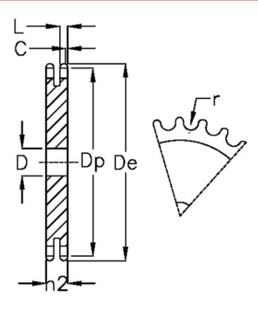
C = 2 D = 25 De = 280.5 Dp = 273.03 For chain size =  $5/8 \times 3/8$ For chain type = 10 B-2 h2 = 25.5
